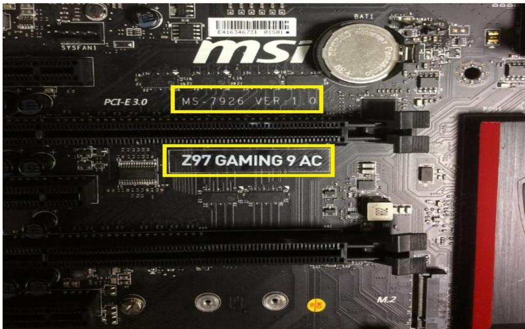
b. Boot up your system & press "delete" key to enter BIOS screen to double confirm BIOS version.
