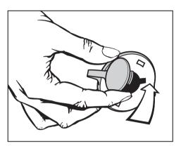
■ Fit the covers on to the two holes. Then plug the holes as shown with the caps.
