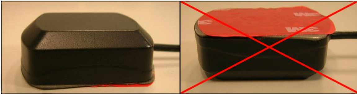
Figure 27 GPS antenna correct mounting.
